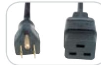
010-9334: NEMA 5-15P to C19 125V, 15A straight blade 8-foot, 14 AWG/3-wire
